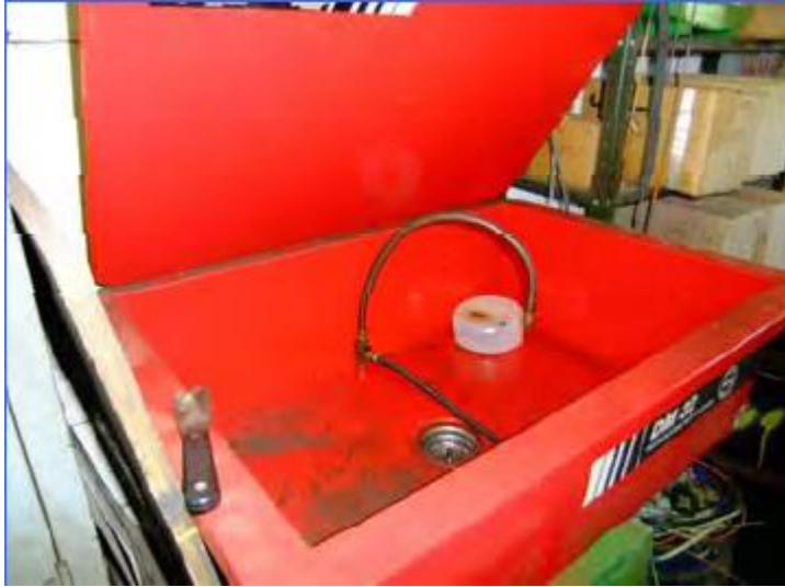
Figure 19: Parts washer in a vehicle maintenance facility. A parts washer should be used to clean parts that have oil or solvents on them. (Hensley, Ann-Drea. 2010. GHP images at Northwest Ohio facilities.
