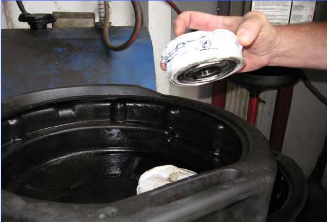
Figure 34: Crushed oil can. Crushing oil cans and recycling oil filters removes excess oil from them and reduces the chance that oil will contaminate streams. (Warren County Public Service Project Group, 2007; Institute of Environmental Sciences.)
