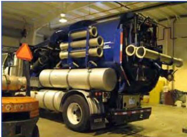
Figure 30: Catch basin vacuum truck. Vacuum trucks pump materials from catch basins to be disposed of in a landfill rather than flushing it into the stream. (Warren County Public Service Project Group-2007. Inst. of Env. Sciences.)
