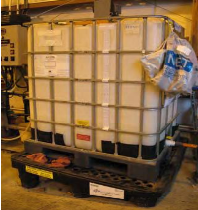
Figure 26: (left) A containment pallet under a liquid storage unit. Containment pallets are useful in preventing slow leaks from spilling onto the floor or ground. They are not useful for large breaches in primary containers. (Warren County Public Service Project Group, 2007. Institute of Environmental Sciences)
